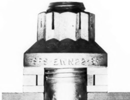
After Preloading. Nut has been tightened down fully. Inner PLI ring has been plastically deformed by compression. Preload in bolt equals force required to deform inner ring.
